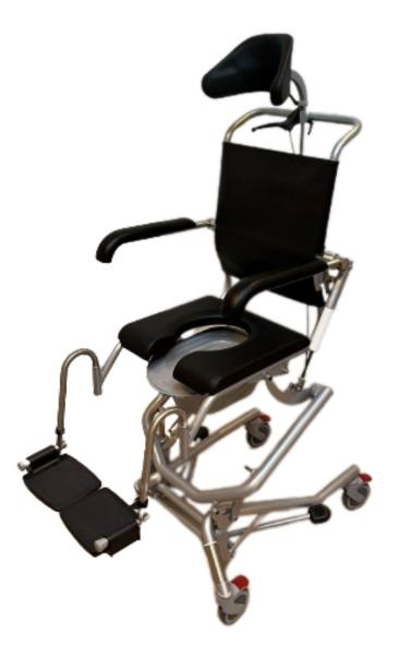
Toilet-shower chair with hydraulic height adjustment and manual tilt via double-acting gas spring.
